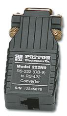
**Note:** Model # 222N9FT (shown above) comes with thumbscrews. Other 222N models come with slotted captive fasteners.
