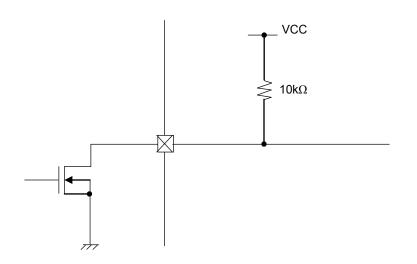
The LO is an open-drain output pin. The LO pin needs to be pulled up to 3.3V/5.0V level for proper function. During regular operation, the LO pin level will stay High (internal MOSFET=OFF). When error detection (TSD, ISD) is applied, the LO pin will show Low (internal MOSFET=ON) level.
