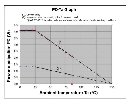
\* This value is dependent on a substrate pattern and mounting conditions. Please be careful. Moreover, power dissipation becomes small when ambient temperature is high.
