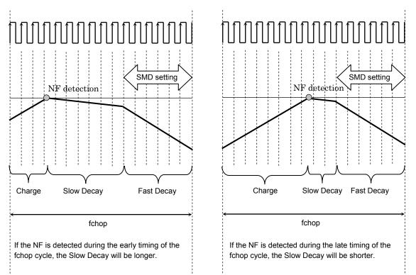
The Charge period is determined by the operating status. Therefore the NF detect timing with in the chopping cycle will change. If NF is detected in the early period of the fchop cycle, the Slow Decay will be longer. If NF is detected in the late period of the fchop cycle, the Slow Decay will be shorter, as shown above.
