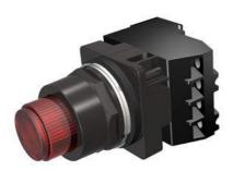
30mm BlackMax, Epoxy Coated Corrosion Resistant Complete Metal Unit PTT / Illuminated Pushbutton Full Voltage, 24V AC/DC Incandescent Lamp Extended Button Plastic Lens, Red 2 Position Momentary with 1 N.O. - 1 N.C. Heavy Duty Contacts, A600/P600 UL Listed, CSA Certified NEMA 1,3,3R,4,4X,12,13 & Automotive Standards
