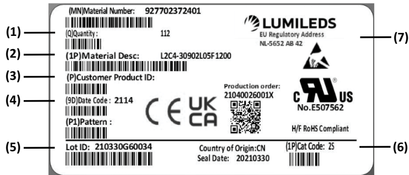
Figure 12. Example of a tray, MBB bag, and inner box label for LUXEON CX Plus CoB (Gen 2).
