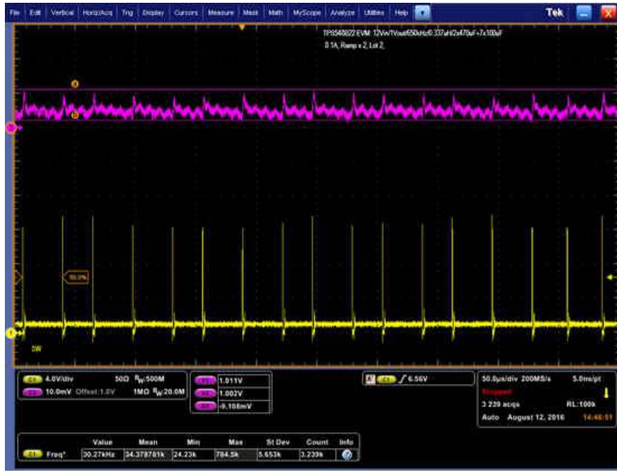
Figure 11-11. Output Ripple and SW Node of 1-V Output at 12 V IN , 0-A Output
