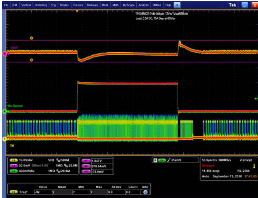
Figure 11-9. Transient Response of 1-V Output at 12 V IN , Transient is 0.5 A to 15.5 A, the Step is 15 A at 40 A/μs
