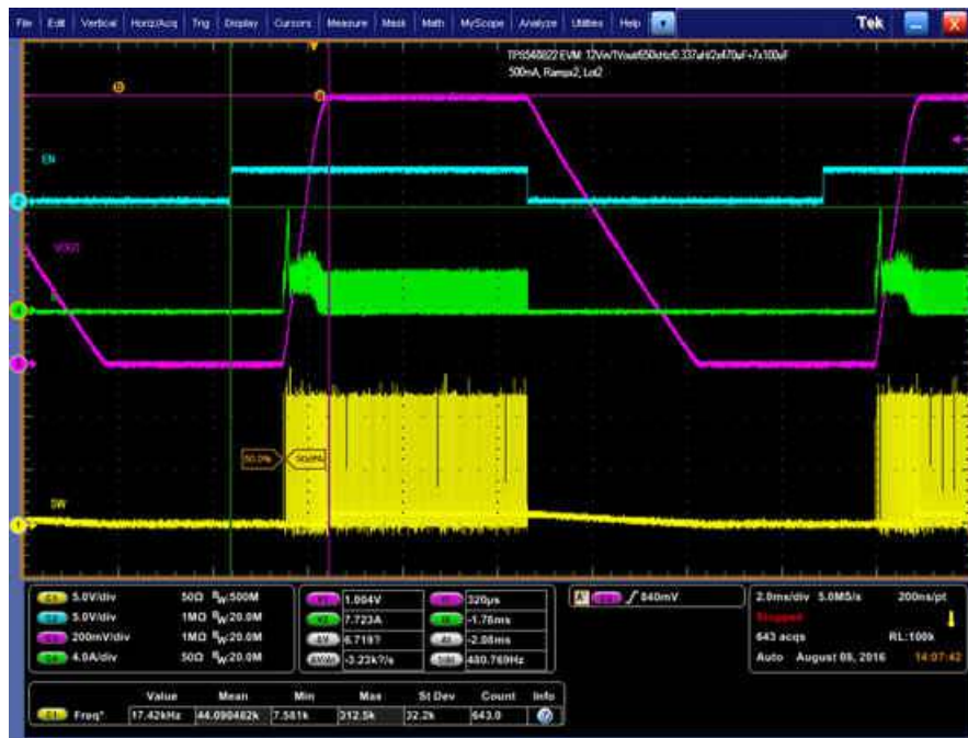
Figure 11-14. Start-Up and Shutdown, 1-V Output at 12 V IN , 0.5-A Output
