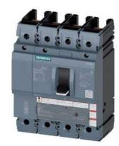
circuit breaker 3VA5 UL frame 250 breaking capacity class C 100kA @ 480V 4-pole, line protection TM210, FTFM, In=175A overload protection Ir=175A fixed short-circuit protection Ii=10 x In N conductor protection 100% without connection
