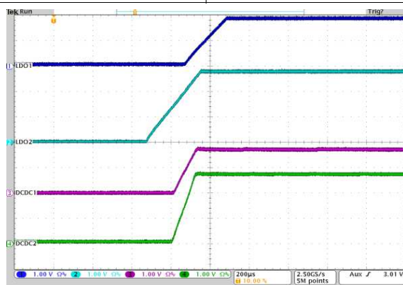
Figure 4-39. Startup DCDC1, DCDC2, LDO1, and LDO2
