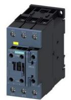
power contactor, AC-3e/AC-3, 41 A, 18.5 kW / 400 V, 3-pole, 21-33 V AC/DC, 50/60 Hz, with integrated varistor, auxiliary contacts: 1 NC, screw terminal, size: S2, F-PLC-IN
