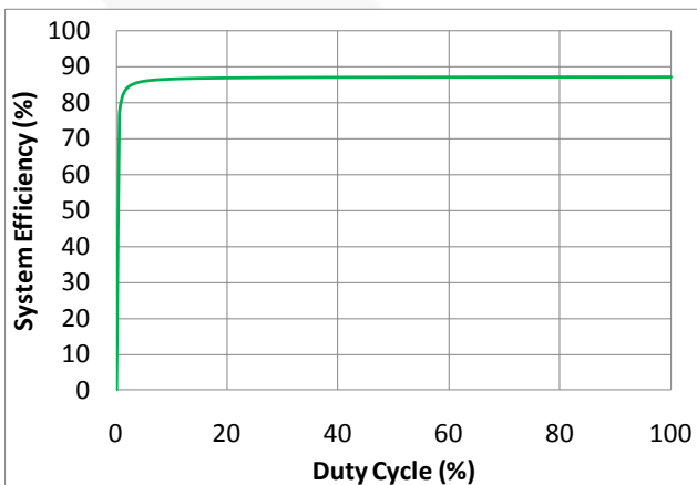
Figure 8. System Efficiency vs. PWM Duty Cycle, f_{PWM} = 1\text{ kHz}
