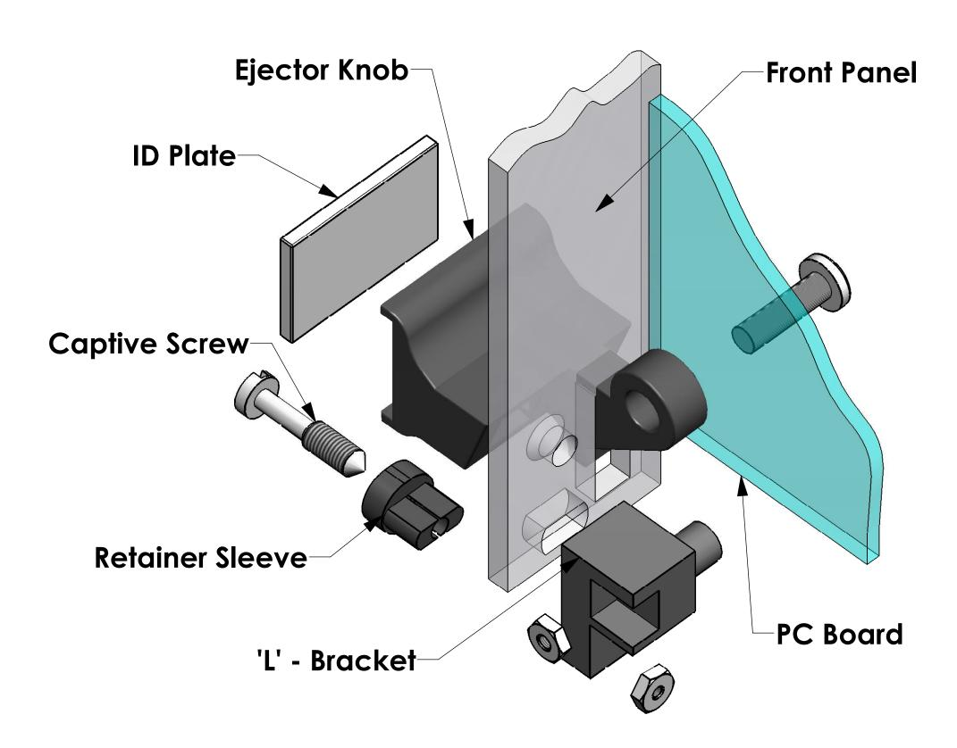
FPE04-6U PANEL WILL HAVE TWO CENTER HOLES FOR OPTIONAL 3U 'L' BRACKETS. ORDER FPE04-6UB FOR PANEL WITHOUT THE CENTER HOLES.
