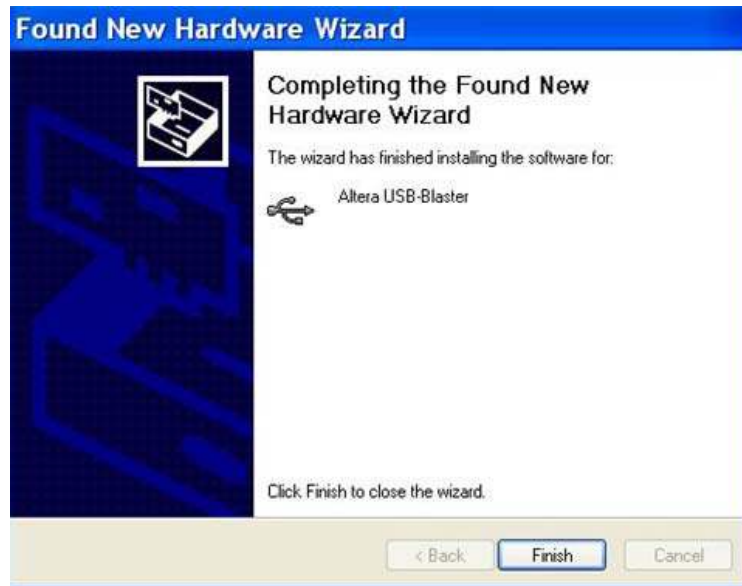
Figure 1-8 The driver is installed
