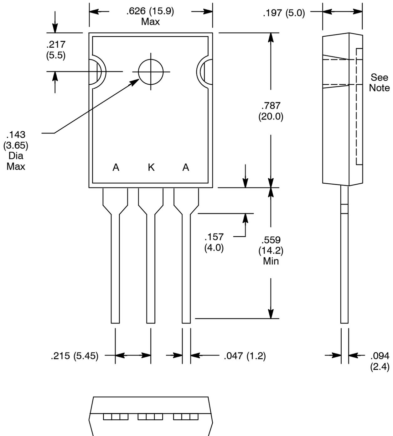
**Note:** Pin2 connected to metal part of mounting surface.
