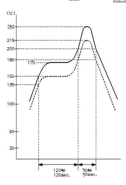
Fig. 3 Reflow Condition
