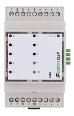
GSM-PRO I/O digital input module, 10 digital inputs 24V with LED display, Mounting type: Mounting rail TS 35, Supply voltage range: 20 V - 28 VDC
