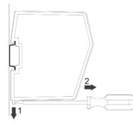
To unmount the module, use a screwdriver to push the DIN-rail fastening mechanism on the back of the module down until it locks in a fixed and open position (1). Then unhook the module from the DIN-rail (2).
