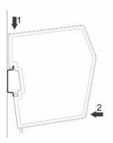
Ensure that the DIN-rail fastening mechanism on the back of the module is in a fixed and closed position, i. e. that it is pushed all the way up.
