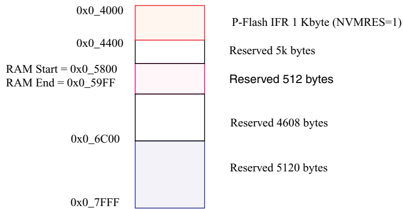
Figure 25-3. Memory Controller Resource Memory Map (NVMRES=1)
