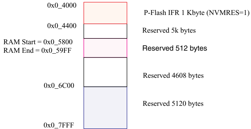
Figure 24-3. Memory Controller Resource Memory Map (NVMRES=1)
