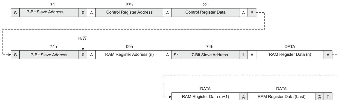
Figure 5-34. Reading from Multiple RAM Registers
