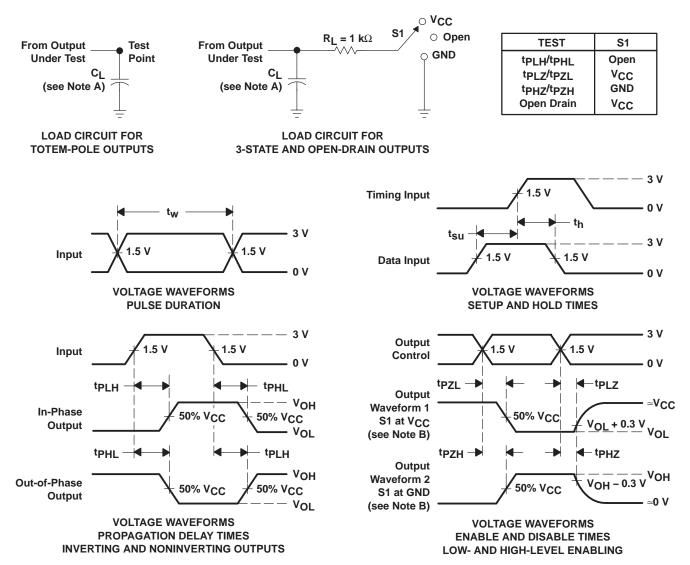
NOTES: A.  $C_I$  includes probe and jig capacitance.
