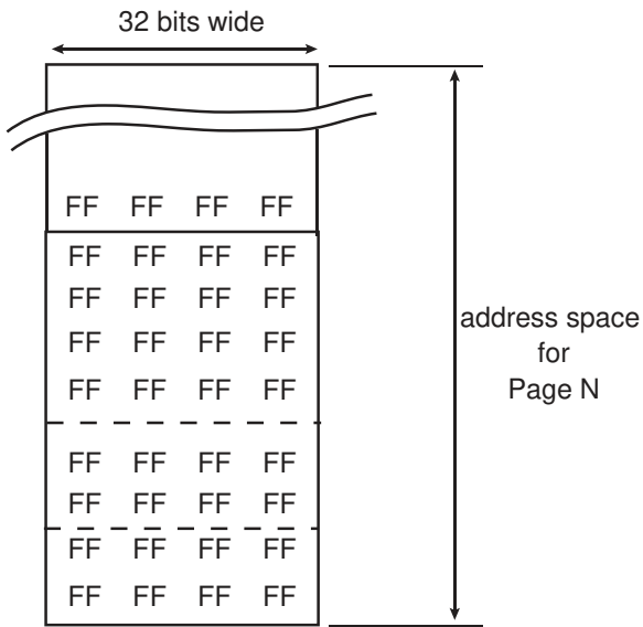
Step 1: Flash array after page erase
