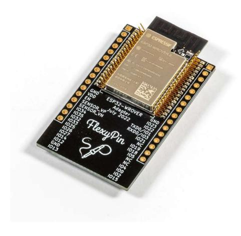
This board allows you to use various modules with a breadboard (and more) without having to solder the module in place. Just add FlexyPins
