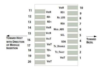
Pin-out of connector Block on Host board
