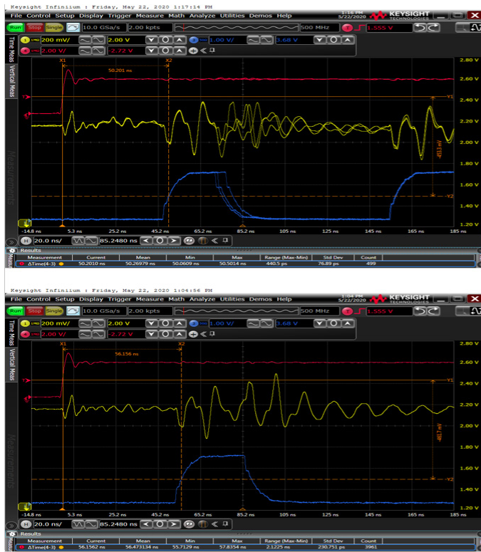
Figure 46. Actual Measurements of Discriminator Circuit at 5 V and 15 V Laser Bias
