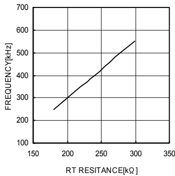
Figure 22. RT resistor vs. oscillation frequency
