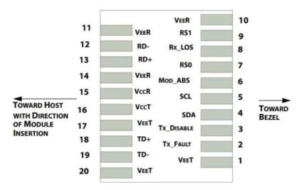
**Electrical Pin-out Details for SFP**
