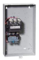
Non-reversing motor starter, Size 3 1/2, Three phase full voltage, Solid-state overload relay, OLR amp range 50-200A, Non-combination type, Enclosure type 1, Indoor general purpose use, Standard width enclosure
