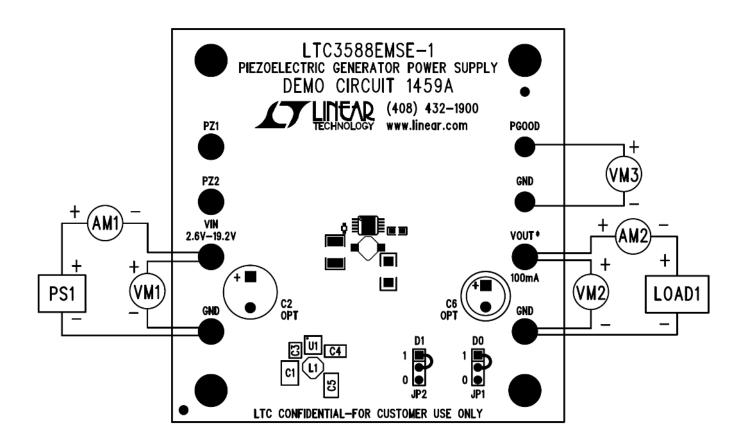
Figure 1. Proper Measurement Equipment Setup
