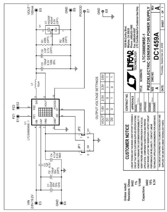
Figure 2: Schematic diagram
