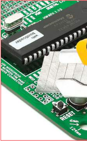
Figure 3-2: cutting copper between pads
