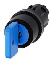
Key-operated switch O.M.R, 22 mm, round, plastic, lock number 73038, blue, with 2 keys, 3 switch positions I-O<II, left latching, right momentary contact type, actuating angle 2x45°, 10:30h/12h/13:30h, key removal O, with laser labeling, lower case
