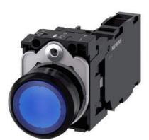
Illuminated pushbutton, 22 mm, round, plastic, blue, pushbutton, flat, momentary contact type, with holder, 1 NO+1 NC, LED module with integrated LED 24 V AC/DC, screw terminal
