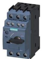
Special type Circuit breaker size S00 for motor protection, CLASS 10 A-release 9...12 A N-release 163 A screw terminal Standard switching capacity with transverse auxiliary switches 1 NO+1 NC Ambient temperature -50 °C 500 switching cycles
