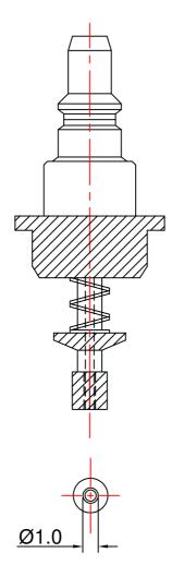
Nozzle Diameter: Ø1.0mm; Please don't blow the acoustic port directly.
