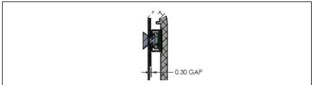
Figure 7-16. Stereo Depth Module Air Gap
