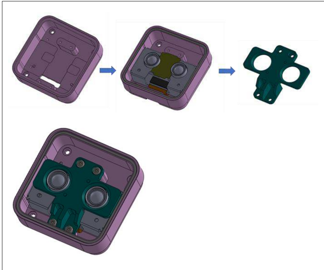
Figure 7-15. Stereo Depth Module Mid-Mounting – D401
