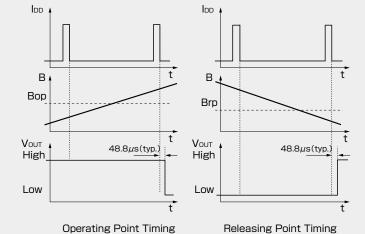
This Hall effect IC's output is held as internal data just before the internal circuit 38 turns OFF (IDD OFF). And after 48.8  $\,\mu$  s, the output changes.
