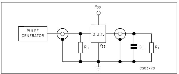
$C_L$  = 50pF or equivalent (includes jig and probe capacitance)  $R_L$  = 200K $\Omega$   $R_T$  =  $Z_{OUT}$  of pulse generator (typically 50 $\Omega$ )
