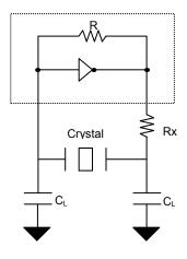
$$\begin{split} C_\text{L} &= 2^*(C_P - C_S), \\ \text{Where } C_P &= \text{Load capacitance of crystal} \\ C_S &= \text{Stray capacitance due to } C_\text{IN, } \text{PCB, } \text{Trace etc.} \end{split}$$
