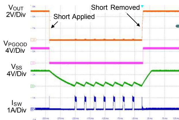
Figure 3. Short Circuit Protection and Recovery
