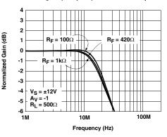
Inverting Frequency Response (Gain)
