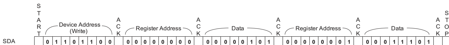
Figure 6: I 2 C Transfer Protocol for Example 2.
