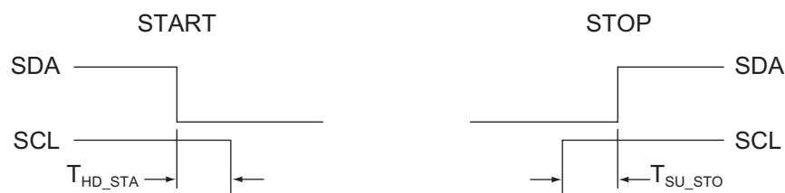
Figure 2: I²C Start and Stop Conditions;
