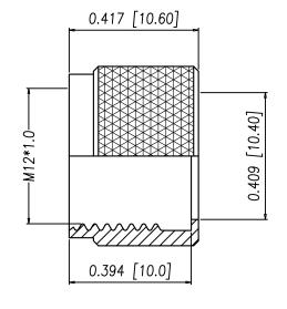
NOTE: MATERIAL HOUSING: PA66 UL94V-0, BLACK CONTACT: **BRASS** NUT: **BRASS** □-RING: EPDM SHELL: **BRASS** FINISH CONTACT: 10u" GOLD PLATED **OVER NICKEL** NICKEL PLATED NUT: SHELL: BRIGHT TIN PLATED **ELECTRICAL** RATED CURRENT: 16A RATED VOLTAGE: 63V WATER PROOF: IP67 WIRE AWG: 14 AWG MAX **ENVIRONMENT**
