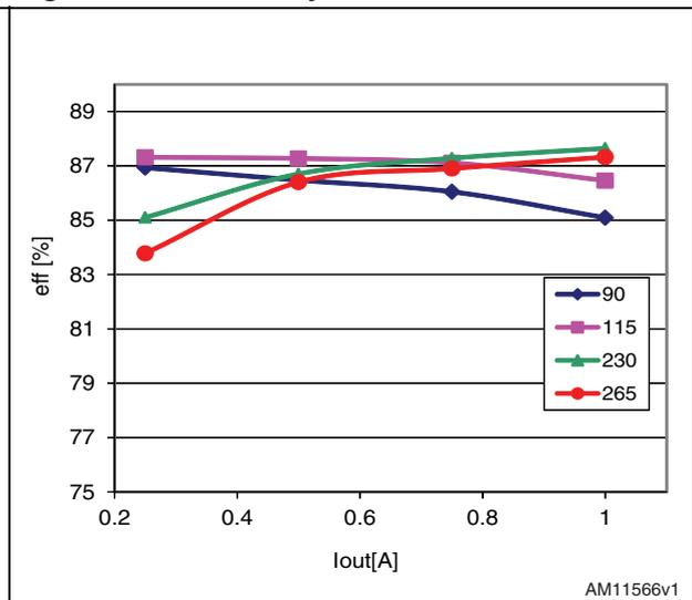
Figure 7. Active mode efficiency vs.  $V_{IN}$
