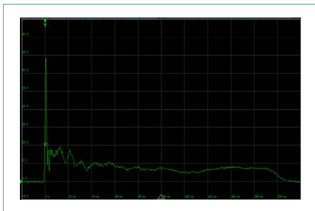
IEC 61000-4-2 +8 kV Contact ESD Clamping Voltage
