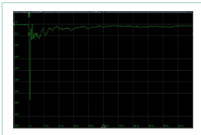
IEC 61000-4-2 -8 kV Contact ESD Clamping Voltage
