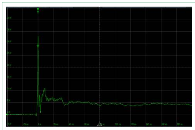
ISO10605 contact discharge plot at +8 kV
