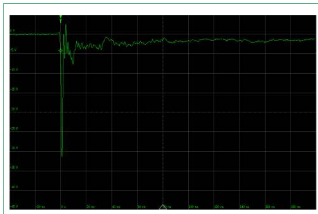
ISO10605 contact discharge plot at -8 kV
