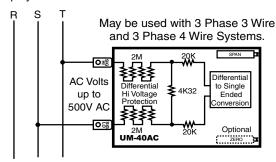
The unique differential input allows safe phase to phase AC line voltage measurements up to 500V AC.
