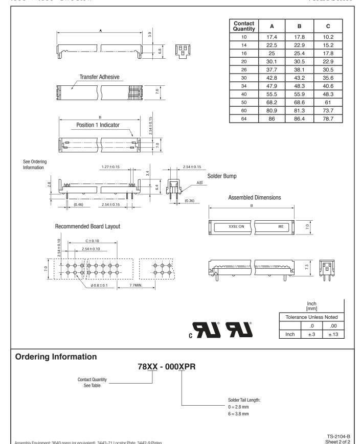
Assembly Equipment: 3640 press (or equivalent), 3443-71 Locator Plate, 3442-9 Platen.
