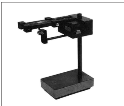
Cable distribution jig
