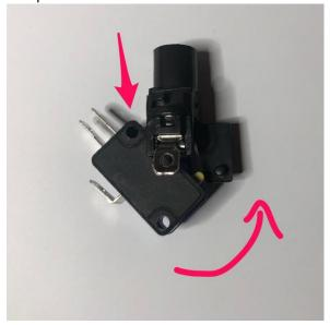
Push the quick connect receptacles onto the blades. The larger ones (0.250") attach to the LED blades, the smaller ones (0.187") attach to the switch blades. Note that COM is the blade on the bottom of the switch, and you can choose whether to attach the second one to either NO (normally open) or NC (normally closed).
