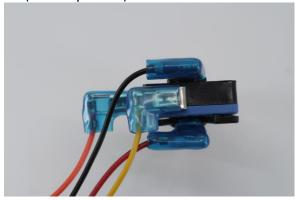
Place the LED into the LED holder, and make a note of which leg the flat side/cathode of the LED is contacting. You'll need to know this later when connecting the button to your project.
