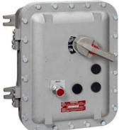
Non-reversing motor starter, Size 3, Three phase full voltage, Solid-state overload relay, OLRelay amp range 25-100A, 110 120/220 240VAC 60HZ coil, Combination type, 100A non-fusible disconnect, Encl. NEMA type 4X Fiberglass Water/dust tight noncorrosive, Standard width enclosure
