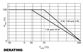
Maximum dissipation ( $P_{max}$ ) in percentage of rated power as a function of ambient temperature ( $T_{amb}$ )
