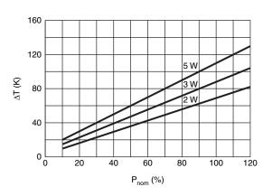
The temperature rise at the solder spot as a function of dissipated power
