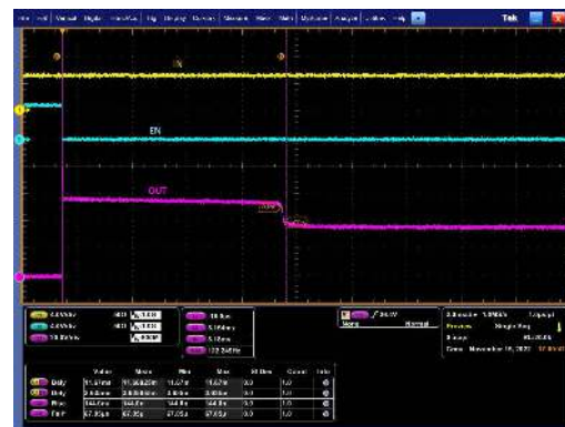
Figure 9-5. OUT In Current Fault Auto Recovery, High Side Mode
