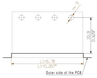
Hole pattern using MPS 5 without middle flange lever
