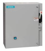
2-speed 3-phase motor starter, Size 0, Two separate windings, Constant or variable torque, Solid-state overload relays, Low Spd OLR range 0.75-3.4A, High Spd OLR range 0.75-3.4A, 110V 50Hz / 120V 60Hz coil, Combination type, 30A disconnect switch, Enclosure NEMA type 4/12, Water/dust tight for outdoors
